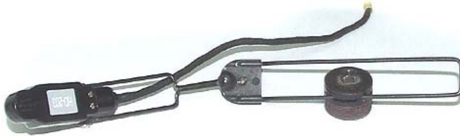
Picture 2. One side of the wire boom removed from the mount.
