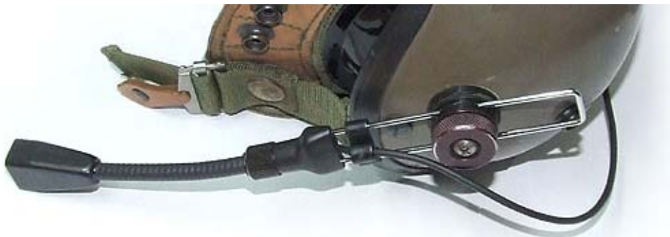
Picture 5. The new boom mounted on the helmet.
