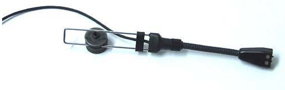
Picture 4. The first side of the boom fitted to the mount.
