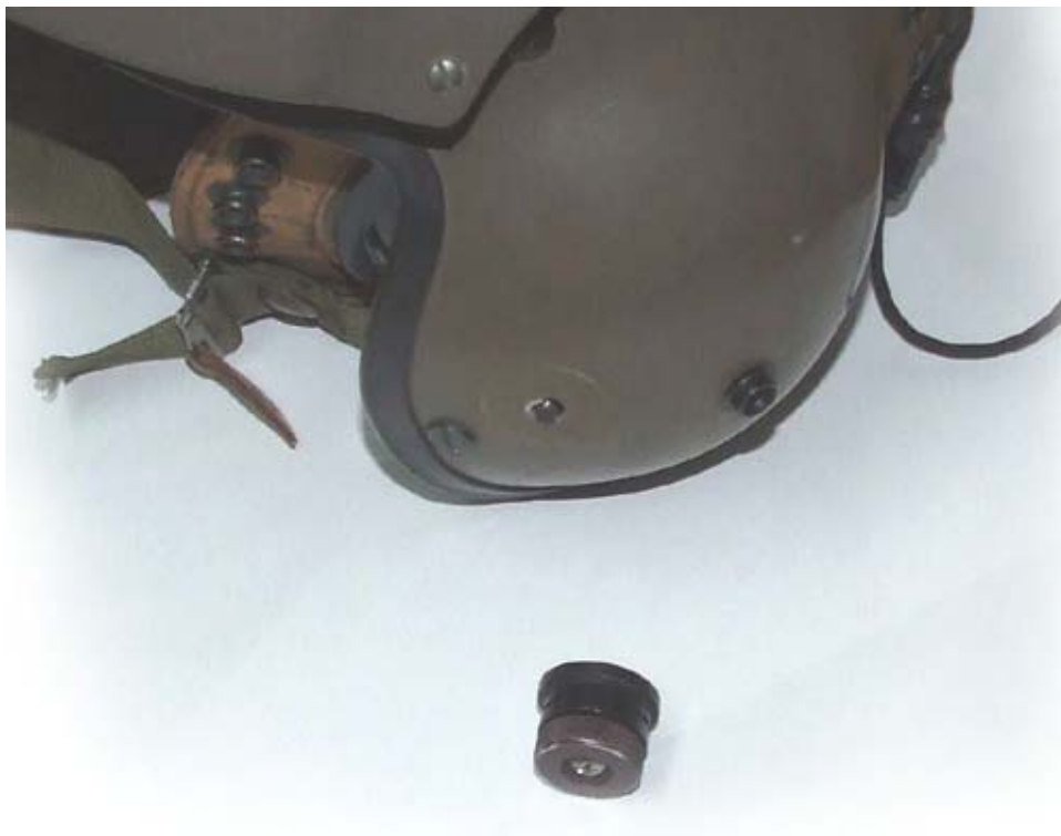
Picture 3. The boom mount ready for fitting of the new boom.
