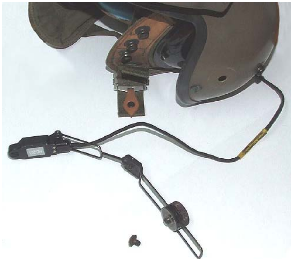
Picture 1 – Wire boom removed from the Gentex helmet
